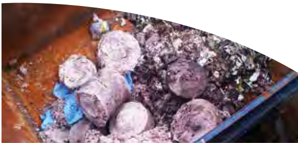
Good quality plug (image results from pumped flow).
