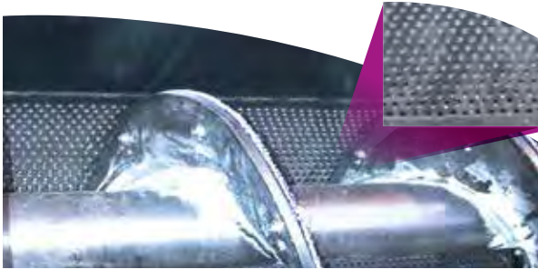
The 9mm thick perforated mild steel trough incorporates 6mm diameter, tapered, holes for efficient fluid discharge.
