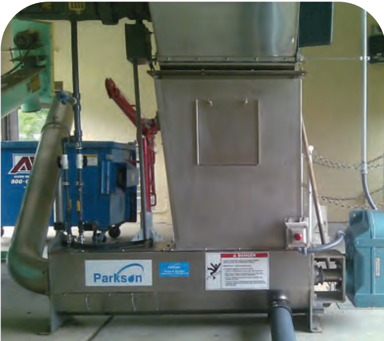
Aqua WashPress® receiving screenings from Aqua Guard® screen
